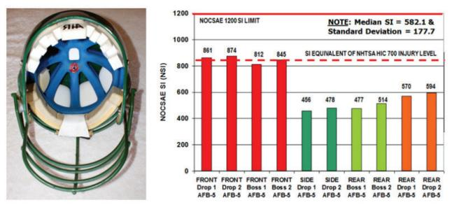
Fig-1. NOCSAE Severity Index Data from 1992 Helmet Design Used by a Fatally Injured High School Player
