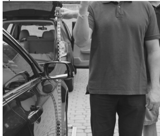
Figure 3: Surrogate demonstrating arm-to-mirror clearance
