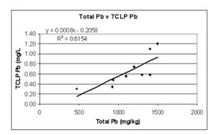
Figure 2: Total Pb versus TCLP Pb using customized (large aliquot) analytical procedures.
