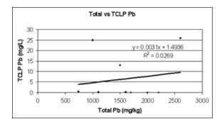
Figure 1: Total Pb versus TCLP Pb using routine analytical procedures.
