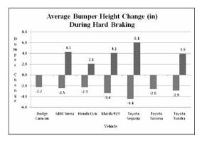
Figure 2: Change in Bumper Height During Hard Braking
